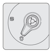
When you turn the valve "\( \overline{\Omega}\)" to the open position, it will start to release steam by itself. Then press the 'quick release button (in the center of the lid)' and the quick release process will start.
