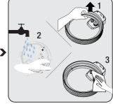
Clean the inside of the lid with water, sealing gasket, steam valve and float can be removed for washing, assemble correctly after washing and dry the inside of the lid with cloth
