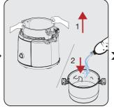
Remove the inner bowl from the housing and place the ingredients and water you will be cooking in it.
