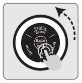
Start the device by pressing the "Start / Cancel" button. Move the adjustment knob to the desired function and press the "Start / Cancel" button again.
