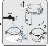
Remove the lid and inner chamber, first clean the chamber with detergent, then rinse thoroughly with water and wipe dry with a soft cloth.
