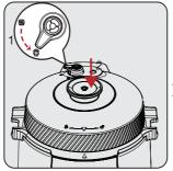
When you want to release steam, turn the valve to the steam open position. The steam will release by itself. If you want to release steam faster, you can release steam manually by pressing and holding the steam release button after turning the valve to the open position.
