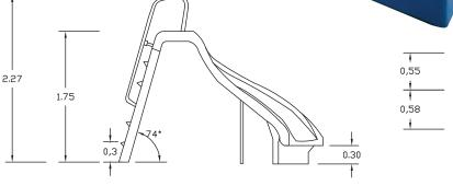
right curved models include 2 water outlets to facilitate downward sliding.
