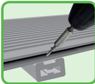
After placing the end clip to each joist as to the middle of the joist, perforate with suitable drill at 45° angle Screw
