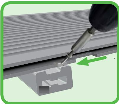
Once you have fitted the final board, mount the final clip in the middle part of each joists and drill the clips using a drill with a bit suitable for 45° angle, then screw the hole you have drilled.
