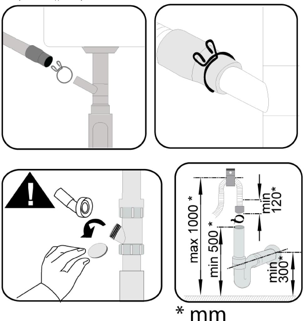
The wastewater drain must be connected to the sewer and must not be connected to surface water.
