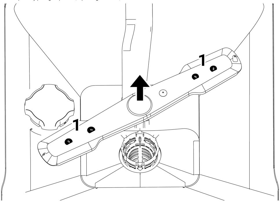
Check whether the holes of the propeller group are blocked. If there is a blockage, remove and clean the impeller assembly. (Depending on model)
