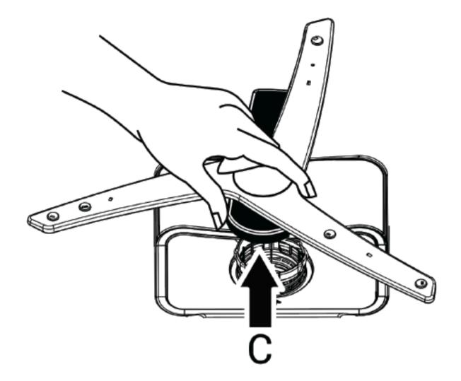
To disassemble and clean the lower impeller group together, remove it by holding it with one hand at the points (C) shown in the figure and pulling it upwards. After the cleaning process, replace the propeller group by performing the same steps in reverse.
