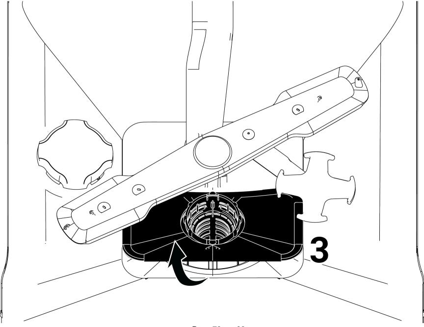
3. Separate the coarse filter from the group by pressing the two tongues on the coarse filter inward.
