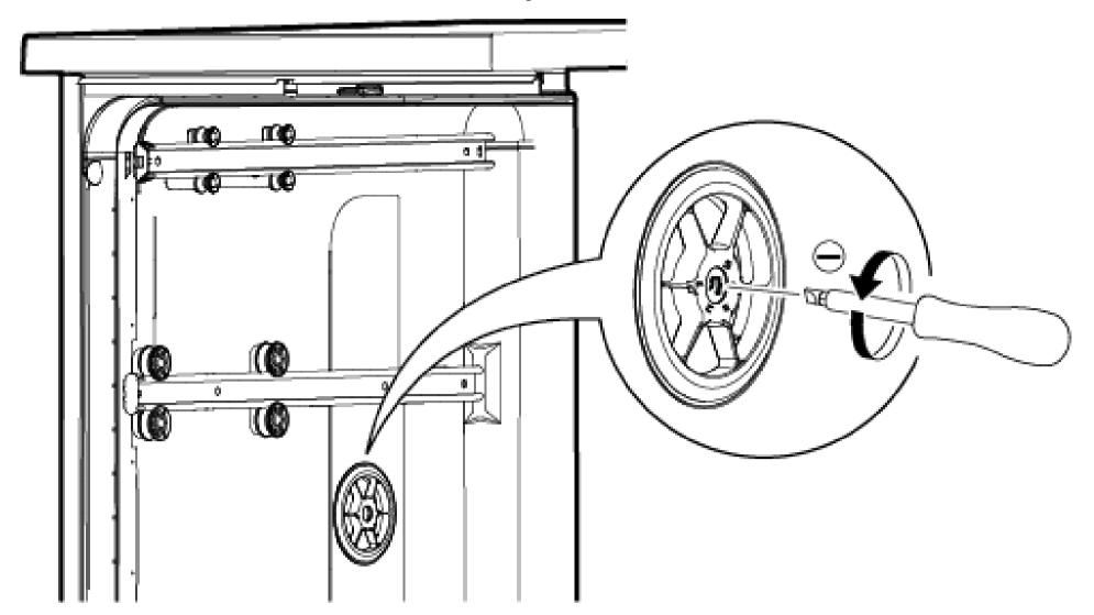
The glass care function setting is used to adjust the water hardness level of the pre-softened washing water in the dishwasher. The setting should be made according to the water hardness adjustment level. Adjustment is made with the help of a wide flat screwdriver. Screwdriver is used to turn the mechanical glass maintenance adjustment switch. Just turn the Mechanical switch to the same position as the water hardness setting level.
