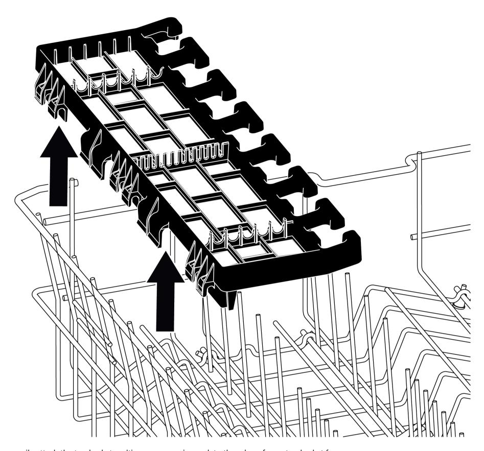
You can easily attach the top basket multi-purpose serving rack to the edge of your top basket for reuse.
