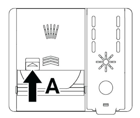
2. Put the specified amount of powder, liquid/gel or tablet detergent into the compartment.
