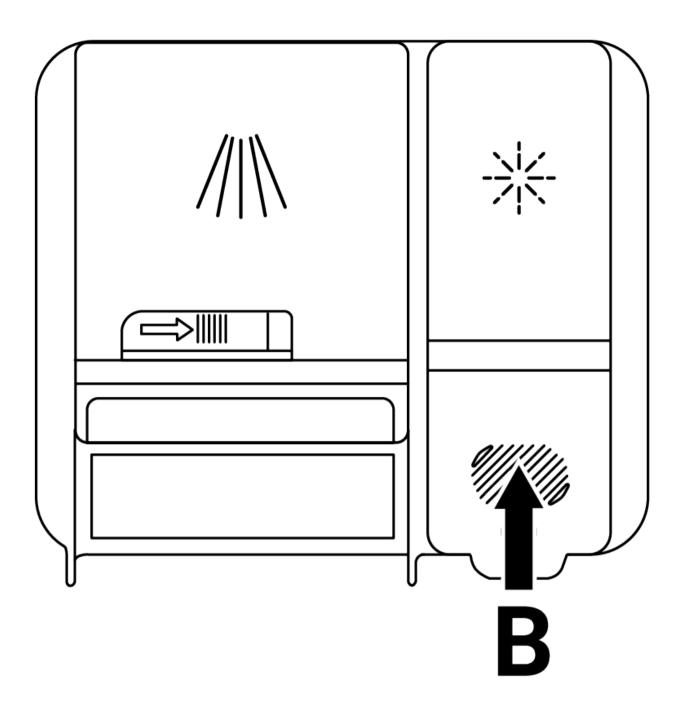
4. If water marks appear on the dinnerware after washing, it is necessary to increase the level of the adjuster, and if a blue trace remains when wiped by hand, it is necessary to decrease it. This setting is set to position 3 at the factory.
