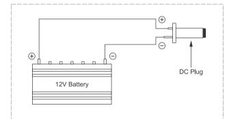
Note: DC Plug is supplied as an accessory with this product, for connecting to the 12V DC Jack provided on the rear of DMX-22. Refer above diagram for making battery cable connection.
