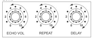
Echo effect is used to repeat the original sound many times to give multiple voice effect and is used for vocals.
