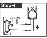
Step-4: Place the speaker on the pole. You can use the supplied pole mount holes larger than 35 mm.
