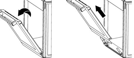
8. Pull the removed door upwards to release it from the right and left hinges and remove it.
