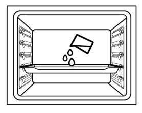
3. Set the oven to the easy steam cleaning operating mode and operate it at 100°C for 15 minutes.
