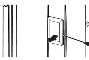
7. Lift the lamp's protective glass cover with a screwdriver. Remove the screw first, if there is a screw on the square lamp in your product.
