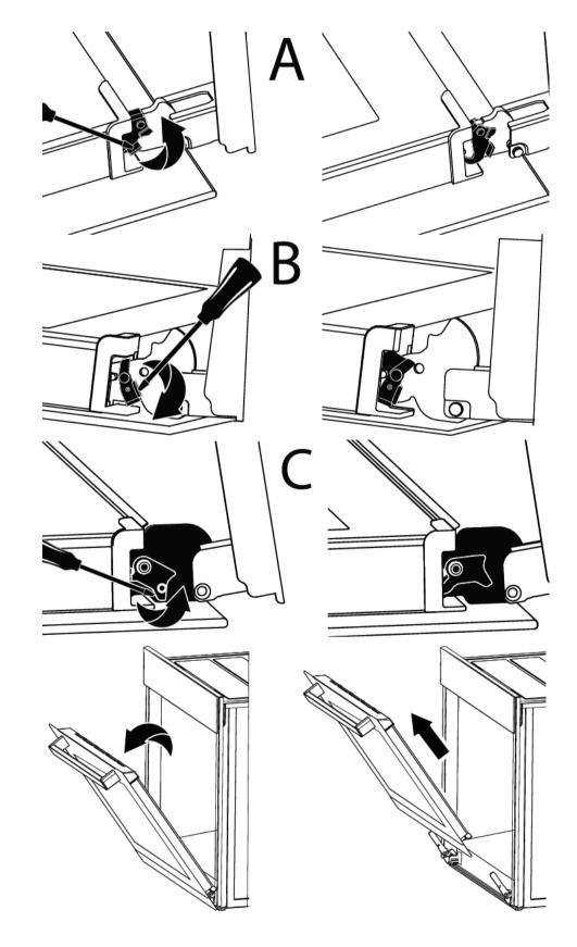
8. Pull the removed door upwards to release it from the right and left hinges and remove it.
