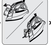
Open the water filling cap (2) and drain the remaining water in the water tank (8) by tilting the appliance forward.
