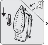
Unplug the appliance before cleaning. Wait for the appliance to completely cool down.
