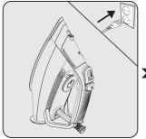
Fill the water tank (8) with water (see 3.3). Set the appliance to the upright position and plug it in.
