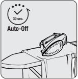
If you do not move the appliance for 30 seconds in lateral position (right or left), it would shut-down automatically.
